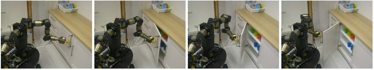
Fig. 3: The robot performing the door opening experiment. v_d = 0.05 m/s. The images are taken at t = 0 s, t = 1.5 s, t = 3.6 s, and t = 5.7 s, respectively.
