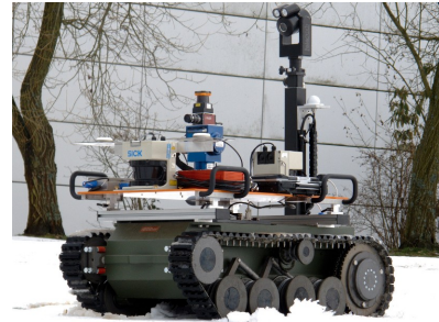
Fig. 1. A Telerob Teodor robot equipped with sensors for basic autonomous navigation.
